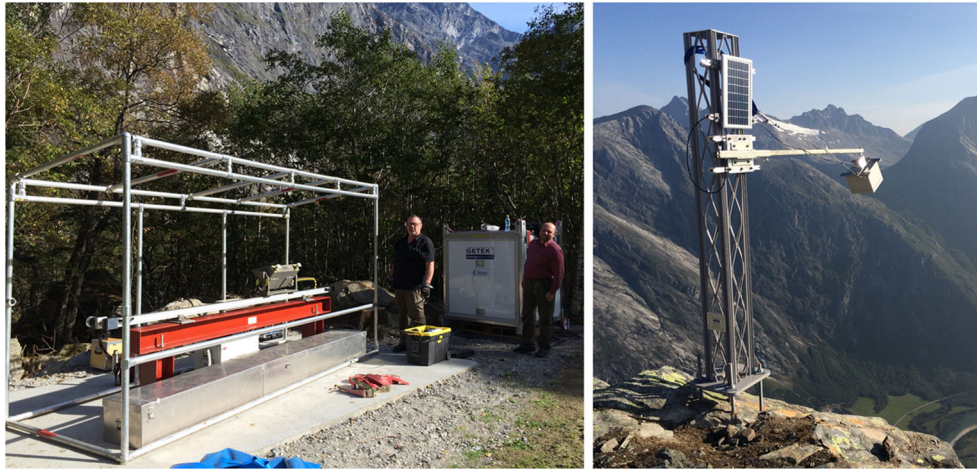
Fig. 4 The GB InSAR system before a permanent hut was built, and a time-lapse camera at the edge of Romsdalen, looking down at Veslemannen
